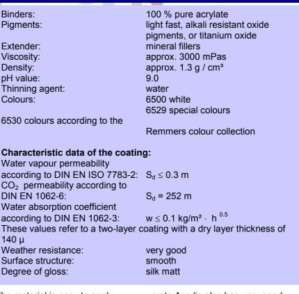
The material is easy to apply. Thanks to its high quality, small, static hair cracks in the substrate are bridged with two coats. Concrete Acrylic also has very good hiding power. Good adhesion to old and new fair-faced concrete as well as restored concrete surfaces
